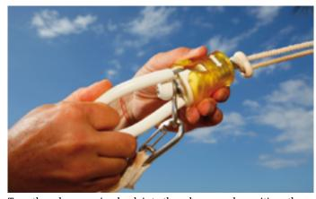
Turn the release casing back into the release ready position, the release casing will snap into the ready position.
