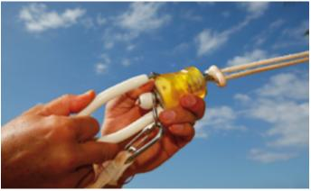
Once the chicken loop ring is threaded over the release stick, place the chicken loop ring into the Rotor release casing.
